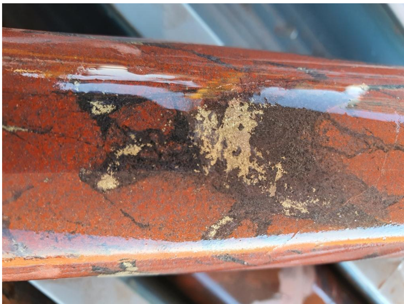
Figure 10 Drill core from drillhole EBD3W2A, approximately 1192m, showing blebby chalcopyrite and red rock alteration.
